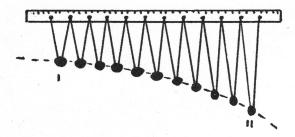
A piece of duct tape encircles each ball and a length of string passes under the duct tape and is attached to the half-metre rule with the bolts, washers and wing-nuts through holes drilled for the purpose. Hence, each ball is supported in such a way that it will swing with no elliptical motion; the length of its supporting string may be easily changed by loosing the appropriate wing-nut. I support the whole thing on any handy shelf or table leg with the C-clamp.
